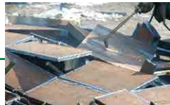
Old thick steel scrap (thickness > 6 mm, < 1.5x0.5x0.5 m)
