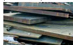
Old thick steel scrap (thickness > 100 mm, < 1.5x0.5x0.5 m)
