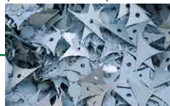
New sheet metal punch scrap (< 1.5x0.5x0.5 m)
