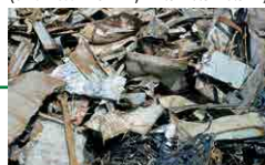
Old thin steel scrap (thickness < 6 mm, < 1.5x0.5x0.5 m)
